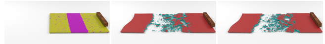
Figure 12: Changing the noise model used to add the impurity within the random graph does not produce much difference in the fracture pattern. Simulated fracture pattern produced when the impurity is generated using Gaussian random variable (middle) and uniform random variable (right).
