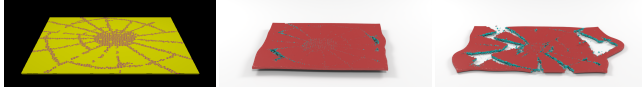
Figure 10: The slab model, embedded with the impurity map created from an image pattern (left), is torn apart by pulling it from both ends (middle, right).
