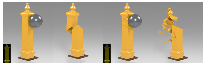
Figure 9: A porcelain column breaks on impact according to the embedded impurity map (inset images) with a single sharp fracture line in the first two images and a more complex fracture pattern in the last two images.
