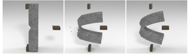
Figure 17: Charpy Impact Test: The left image shows the configuration of the Charpy test. In the middle image, a specimen with a higher plasticity threshold splits into two, while on the right a specimen with a low plasticity threshold only bends and gets partially damaged.
